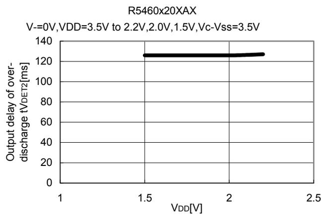
4) Output Delay for Release from Over-discharge vs. V<sub>DD</sub>
