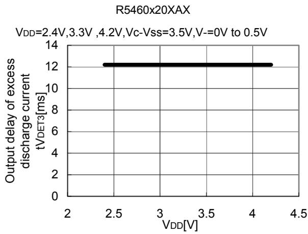
6) Output Delay for Release from Excess Discharge Current Detect vs.  $V_{DD}$
