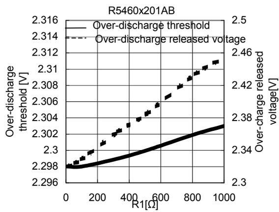
Part 5 Charger Voltage at Released from Over-discharge with a Charger dependence on R2
