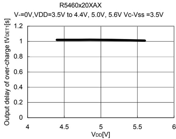
2) Delay Time for Release from Over-charge vs. V<sub>DD</sub>
