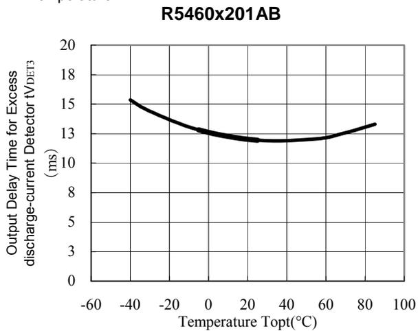
16) Output Delay for Release from Excess discharge-current vs. Temperature
