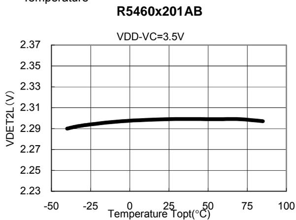
10) Release Voltage from Over-discharge (Cell1) vs. Temperature
