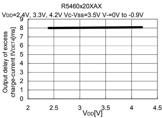
8) Delay Time for release from Excess charge current detect vs.  $V_{DD}$
