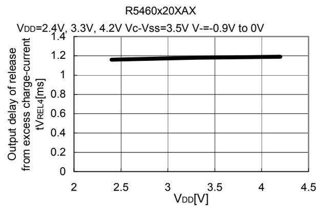
9) Output Delay for Short vs.  $V_{DD}$
