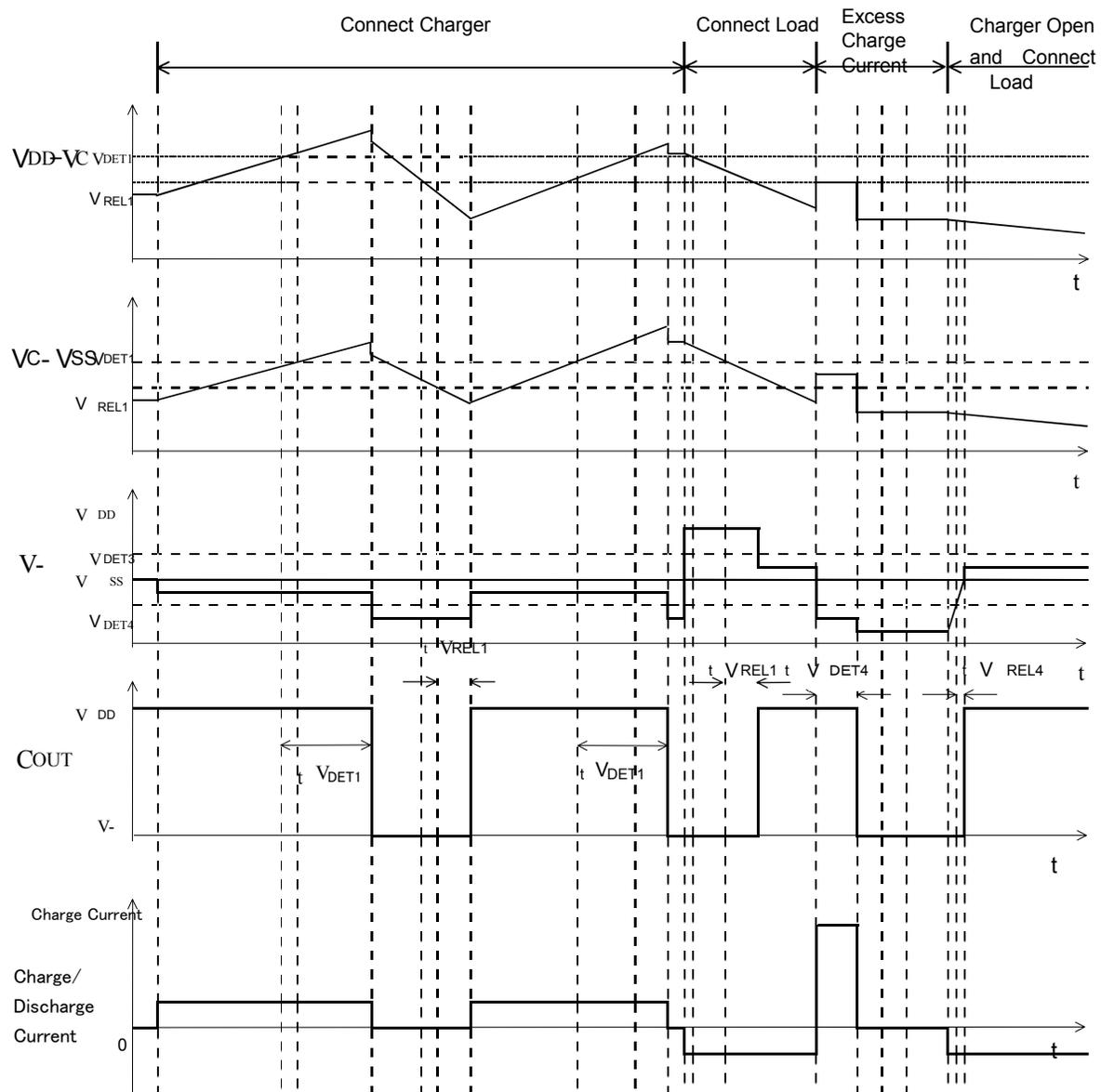
(2) Over-discharge, Excess discharge current, Short circuit
