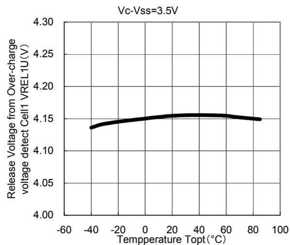
5) Release Voltage from Over-charge (Cell2) vs. Temperature
