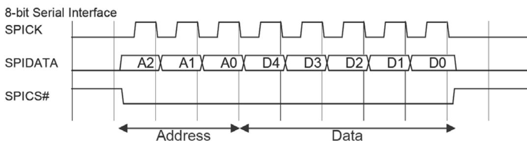
Figure 3 SPI Interface Date Transmission Timings
