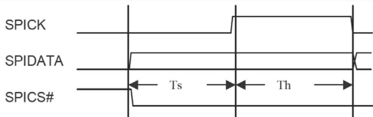
Figure 4 SPI Interface Timing Diagram
