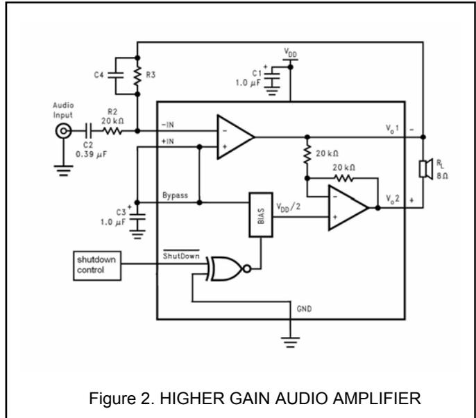
Figure 2. HIGHER GAIN AUDIO AMPLIFIER
