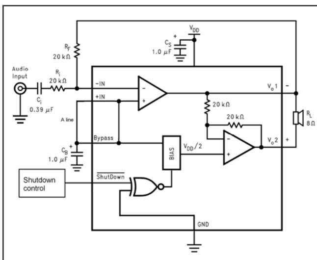
Figure 1. Typical Audio Amplifier Application Circuit (ft690V、ft690M)
