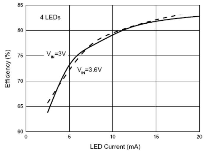
Figure 11. Efficiency vs. LED Current
