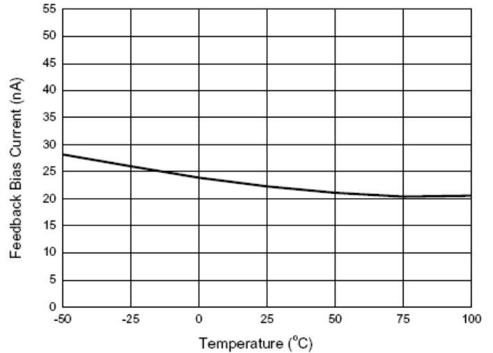
Figure 7. Feedback Bias Current vs. Temperature
