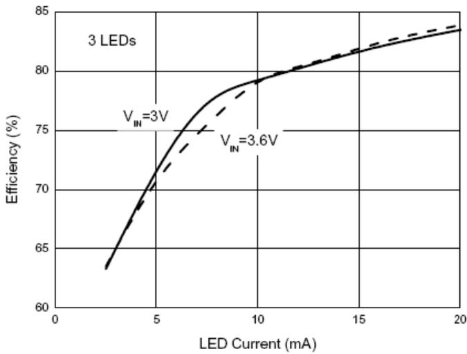
Figure 10. Efficiency vs. LED Current
