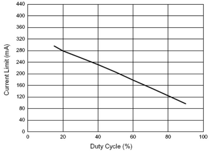
Figure 9. Switch Current vs. Duty Cycle
