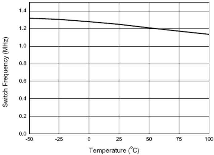
Figure 6. Switch Frequency vs. Temperature
