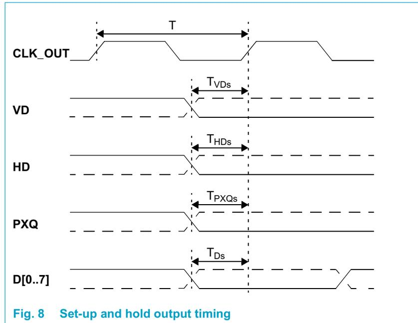
Fig. 8 Set-up and hold output timing
