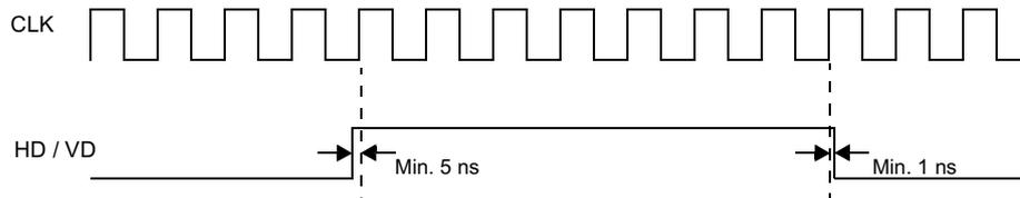
Fig. 6 HD/VD setup timing
