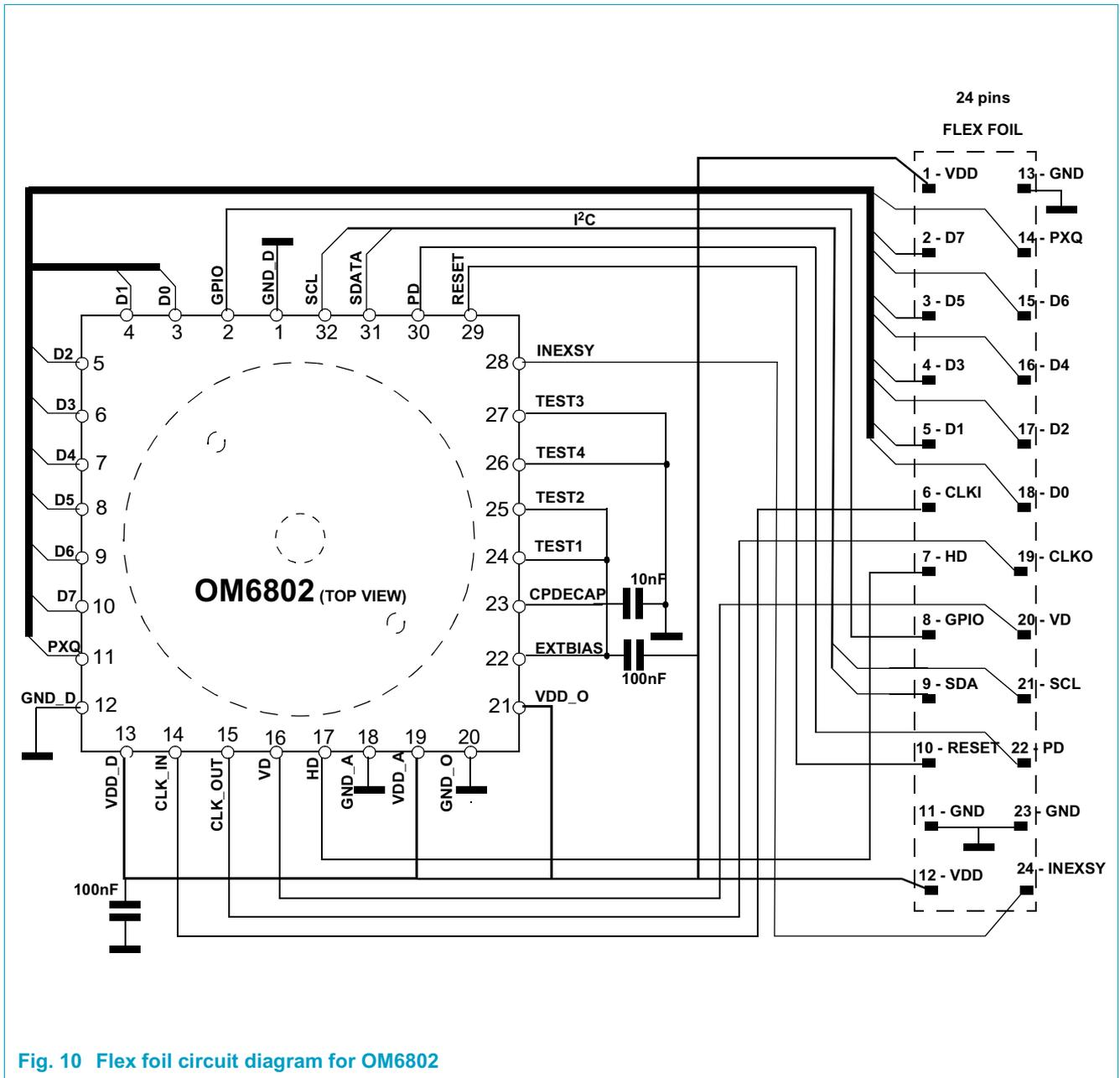
Fig. 10 Flex foil circuit diagram for OM6802
