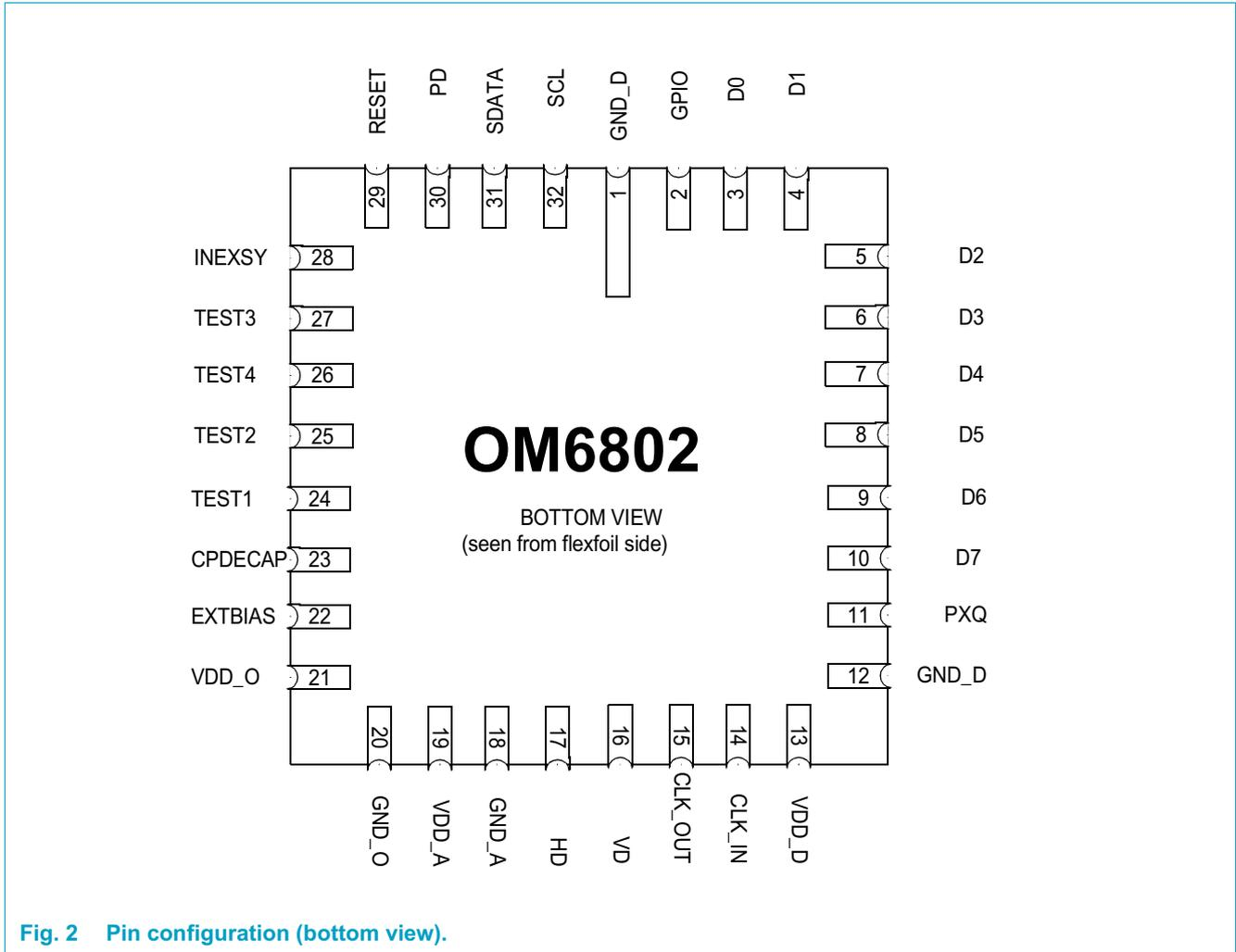
Fig. 2 Pin configuration (bottom view).
