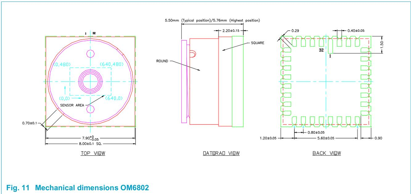
Fig. 11 Mechanical dimensions OM6802
