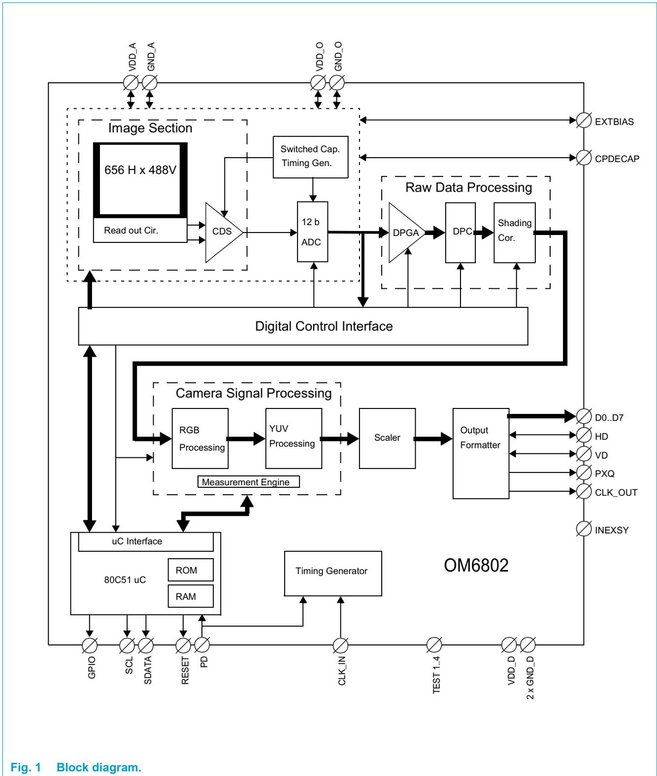
Fig. 1 Block diagram.
