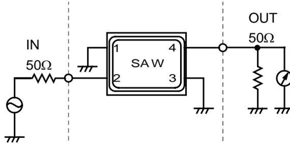
Fig.1 Measuring circuit
