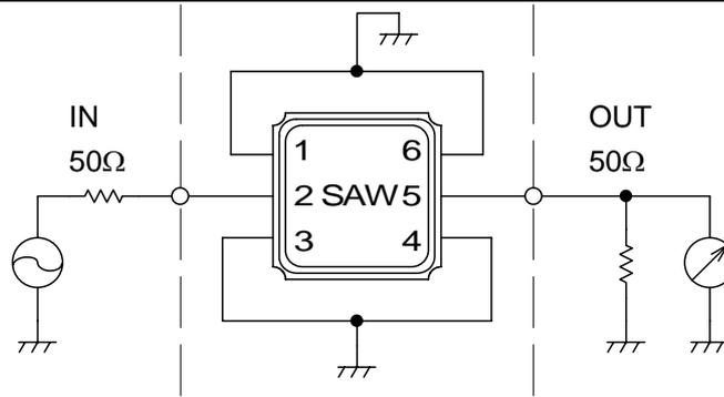
Fig.1 Measuring circuit
