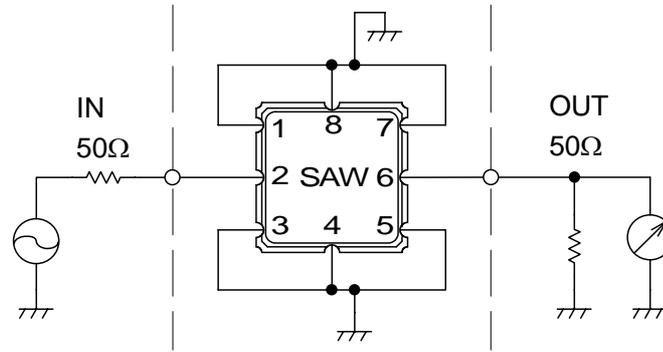
Fig.1 Measuring circuit
