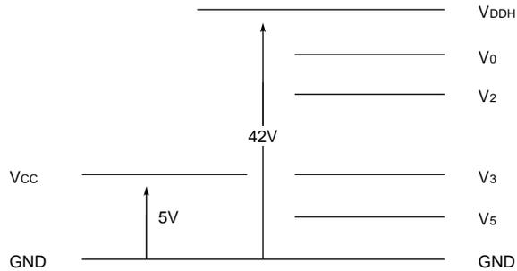
Note 4: Do not allow the logic operation power goes to floating state or V<sub>CC</sub> goes to 2.6V or less while LCD drive circuit power is applied. Otherwise, LSI can be permanently damaged. Special care is needed for the system power on or off sequences.
