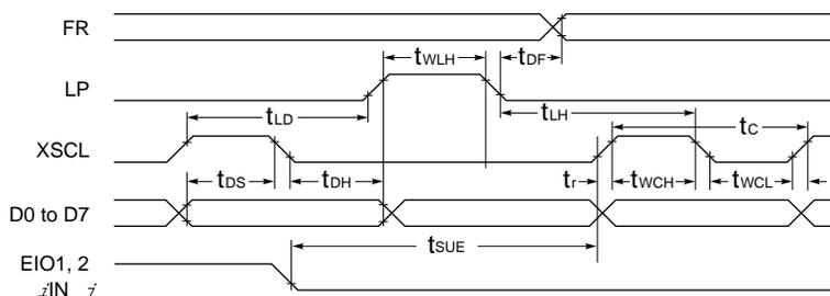
( $V_{CC} = +5.0V \pm 10\%$ ,  $T_a = -30$  to  $85^\circ C$ )
