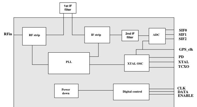
**Figure 1: Block Diagram of RF3000A**
