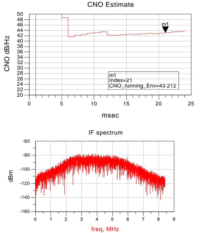
**Figure 11 HP Ptolemy Co-simulation results of noiseless receiver**
