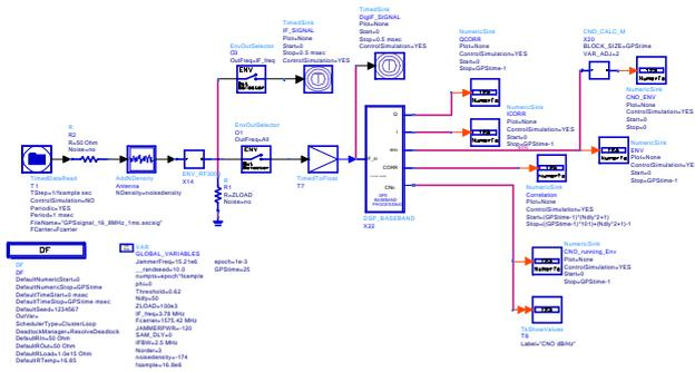
Figure 6 RF3000 HP Ptolemy Co-simulation Schematics
