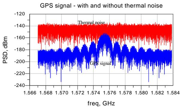
Figure 3 GPS signal spectrum
