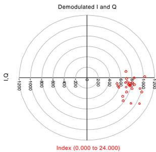
**Figure 10 HP Ptolemy Co-simulation results showing I,Q polar plot**
