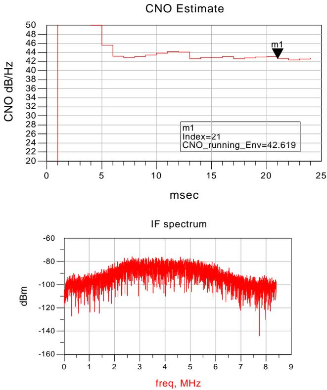
**Figure 9 HP Ptolemy Co-simulation results with no phase noise contributions**
