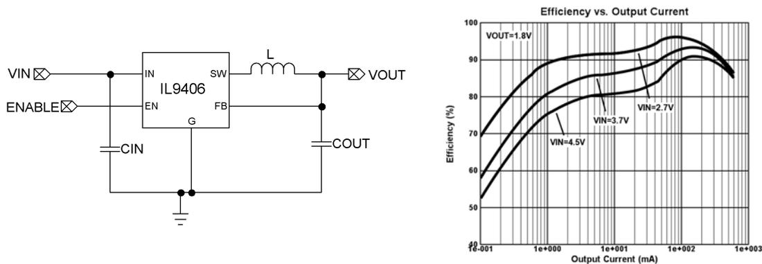
Figure 1. Typical Application Circuit and Efficiency
